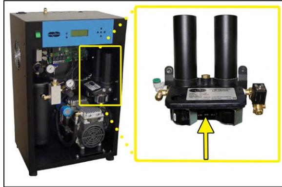
**9.7.2** Use a Voltmeter to measure the DC voltage across each set of “**VALVE**” terminals.
