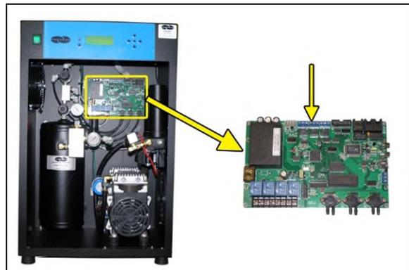
**8.11.3** Wire the Common Alarm wire pair to the Control Board as required:
