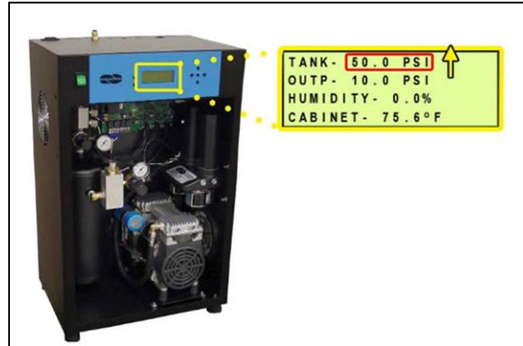
*If the tank pressure (**TANK**) fails to reach 50 PSI (344.7 KPa), see section 13.15 for troubleshooting information.*
