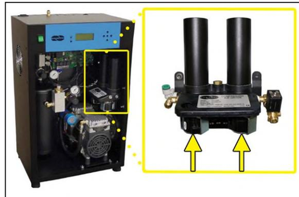
**9.5.4** Place your hand beneath the purge solenoids to feel for purging air. Air should:
