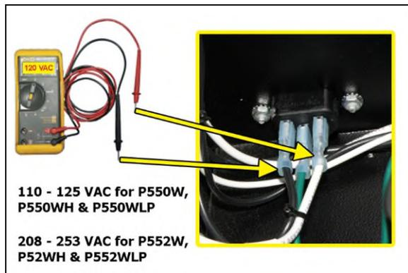
The voltage should measure **110 - 125 VAC** for the BD550W and BD550WLP or **208 - 253 VAC** for the BD552W and BD552WLP.
