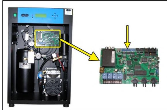
8.12.3 Wire the Power Fail Alarm wire pair to the Control Board as required:
