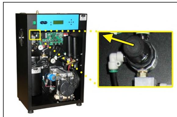
**8.10.3** Turn knob until Outlet Pressure (**OUTP**) reading is at the desired setting.
