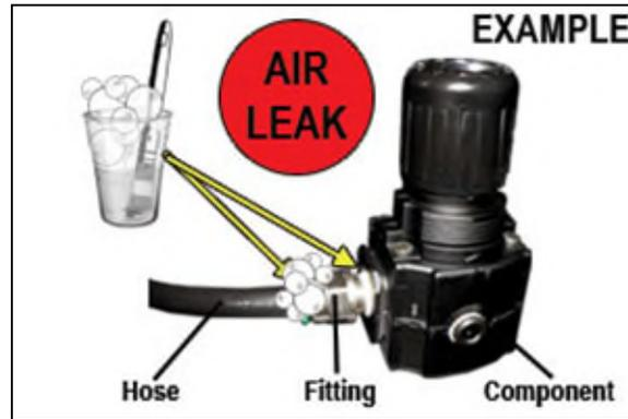
If air bubbles appear at the connection, this indicates that air is leaking from the connection.
