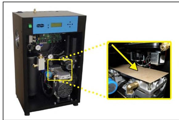
**9.5.3** Locate the heatless Dryer purge solenoids inside the air Dryer
