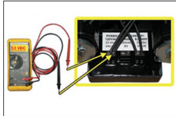
The voltage should measure **53 VDC for 110V units and 106 VDC for 240V units.**
