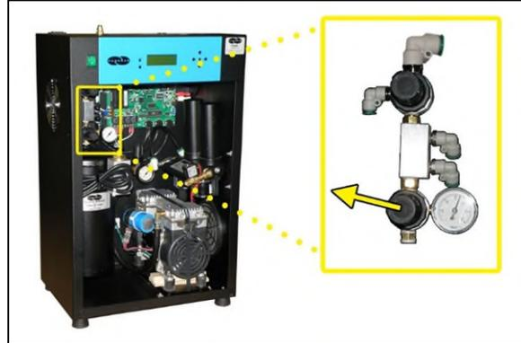
8.9.3 Turn knob until the reading on the Pressure Gauge is **17 PSI (117.2 KPa)**.
