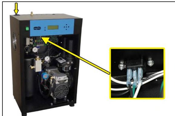
**9.4.3** Use a Voltmeter to measure the voltage (inside Dryer):
