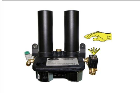
*If air flows from this valve continuously the Unloader Valve is defective and should be repaired or replaced. See sections 11.3 for part detail and 11.7 for ordering information.*
