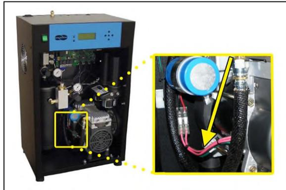
**9.2.3** Use an Amp Meter to measure the running amps.
